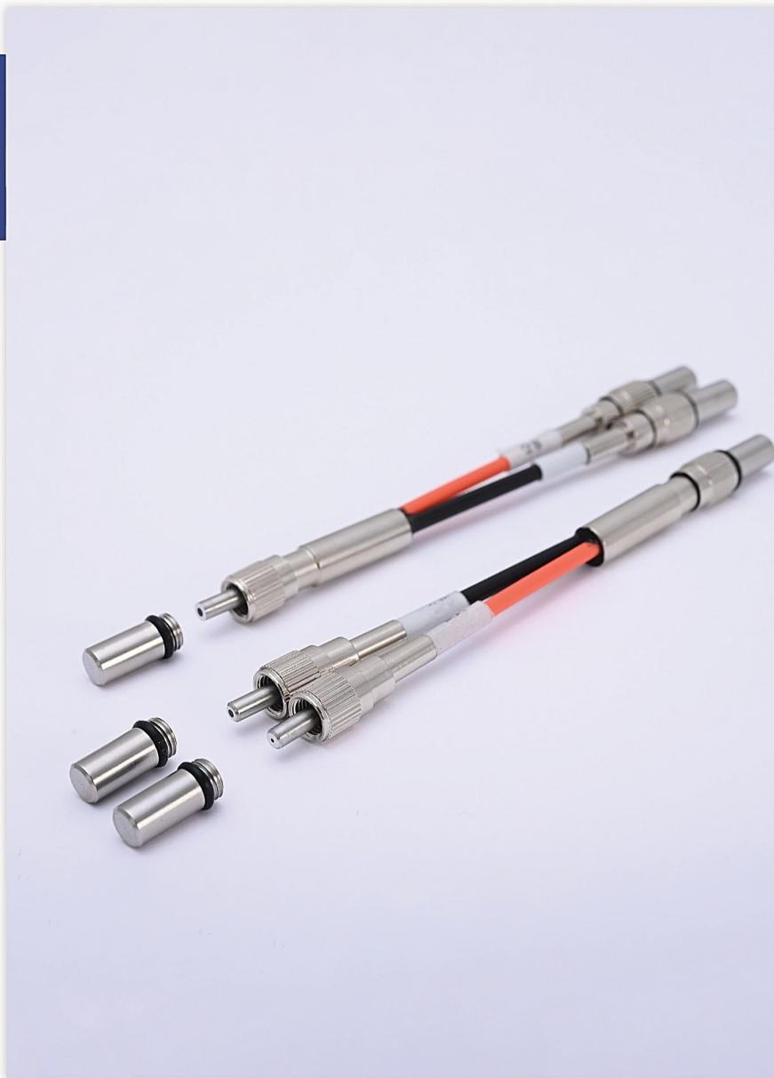
The I2R Labs Dual-Arm Fiber Optic Y-Coupler is a high-precision optical probe designed to split or combine light efficiently for use in reflectance, fluorescence, or dual-source illumination setups. Featuring two independent fiber bundles (SU900/630/600AE.22 and SU600/420/400AE.22) joined into a common SMA905 output, this Y-probe is ideal for biomedical, analytical, and material sensing applications.
