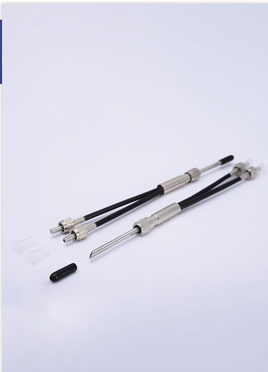
This angled dual-arm fiber optic probe from I2R Labs is designed to enable simultaneous light delivery and collection in compact, field-ready optical setups. Featuring a 38° angled main output tip, the probe enhances targeted reflectance and fluorescence excitation, especially on surfaces or biological samples. The split arms are terminated with SMA905 connectors, allowing easy integration with spectrometers and light sources.
